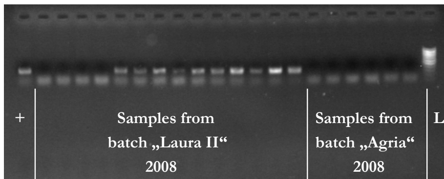
Fig. 2. Image of resolved amplification products on 0.9% agarosis gel stained with ethidium bromide. (L: Low range mass ruler DNA Ladder; +: positive standard e.g. DNA extracted from pure P. infestans mycelium)
