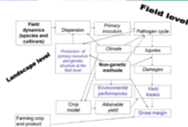
Figure 1. Conceptual framework of SIPPOM, a generic model simulating the effects of cropping systems and their spatial arrangement on epidemics and the durability of specific resistances.
